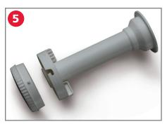
Unlock the base of the sheath and remove the debris collector. Rinse until all non-magnetic debris has been removed. Replace and secure the debris collector onto the sheath and place back into the MagnaClean Professional. Insert the magnet lid assembly and tighten until sealed.
