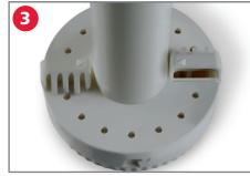
IMPORTANT – Ensure the louvres are in the correct position according to the flow. If the flow enters the bottom inlet, both louvre triangles should point to the sheath stem. If the flow enters the top inlet, both louvre triangles should point away from the sheath stem.
